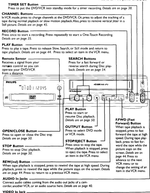
Connect a video cable coming from the video out jack of a camcorder, another VCR, or a video source (laser disc player, video disc player, etc.) here. Details are on page 40.
